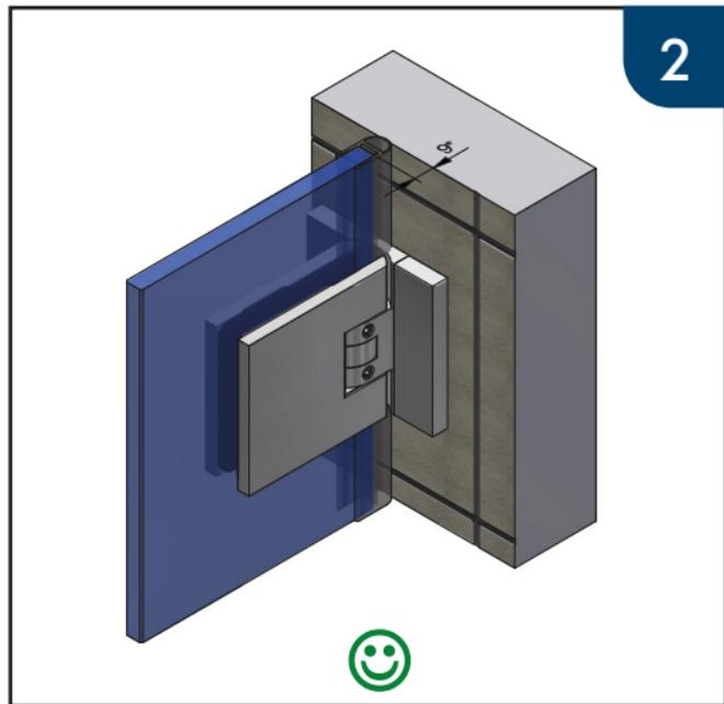
To prevent tilting of the rotational axis, always mount the shower door hinge in such a way, that its entire surface has contact with one tile.
