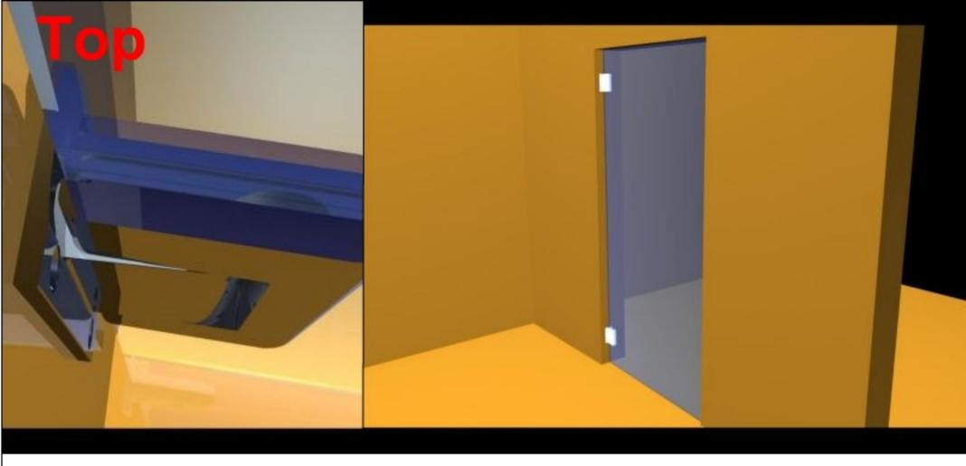
The oil-pressure hinges are supplied with the control valves completely closed (once the door is mounted, it will not in fact be able to close) In order for the valves to function at their best it is necessary that they are well synchronised. To obtain this result it is fundamental to adhere to the following procedure:
