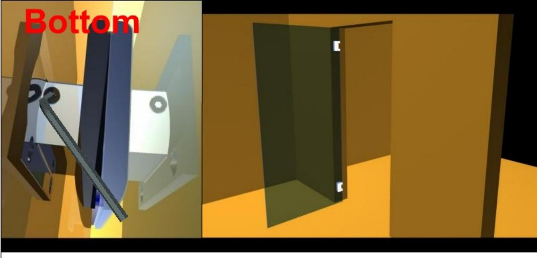
3a) Using the valve control of the bottom hinge, check that the closing speed increases.
