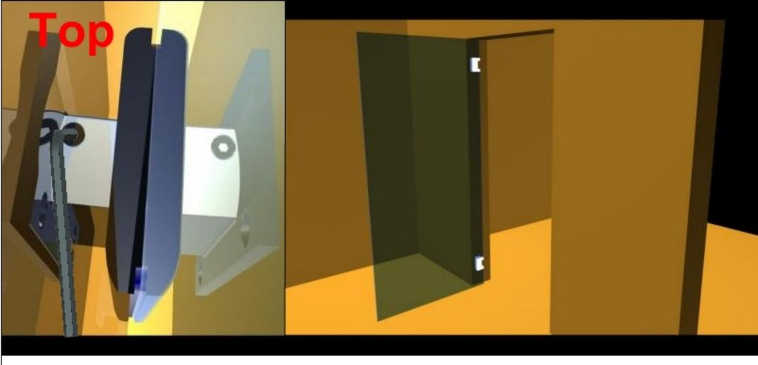
2a) Screw out 1/4 turn the valve of top hinge. Close the door about 10°/15° and make sure that it starts closing automatically.
