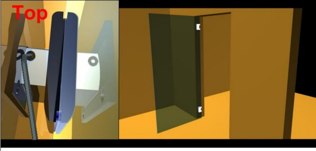
2b) Continue to open or close the valve till you obtain the desired closing speed.
