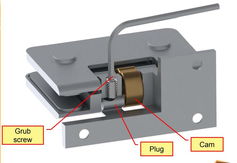
• The grub screw has to be <u>strongly and safety tightened</u>, so that it does not become loose during the normal functioning of the hinge, causing thus the cam movement and the disalignment of the hinge.
