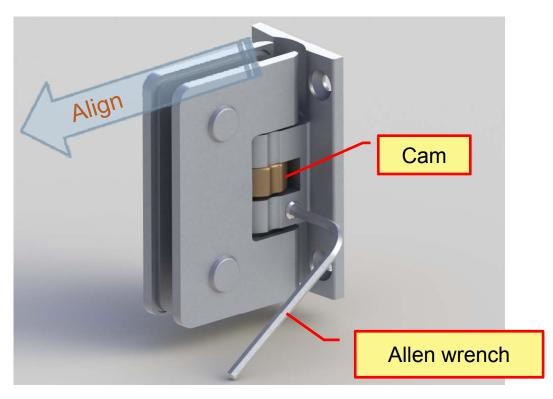
In order to align the hinge 850R we have to position the hinge first, then we have to <u>tighten the grub screw strongly</u> using the allen wrench.
