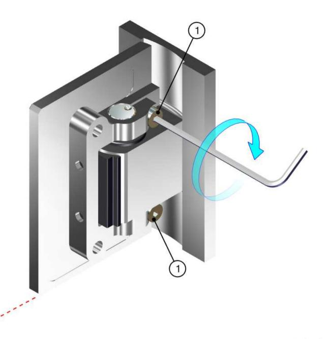
Once the  $0^{\circ}$  is aligned, tighten the screws (1)
