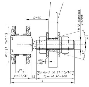
H = Swivel body corresponding to the thickness of the glass.  $V^*$  = glass thickness
