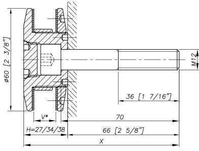
$H\!\!=\!Swivel$  body corresponding to the thickness of the glass.  $V^{\star}=$  glass thickness.
